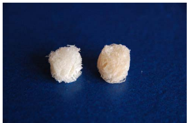
Fig. 1 Picture showing chitin scaffold (left) and chitin/nanosilver composite scaffold (right)
